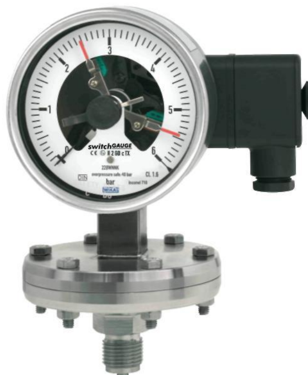
Diaphragm pressure gauge model 432.56.100, high overpressure safety up to 40 bar, with switch contact model 831.21
